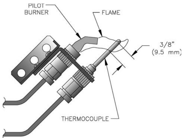
**Figure 24: Typical Pilot Flame, Honeywell Q350**
