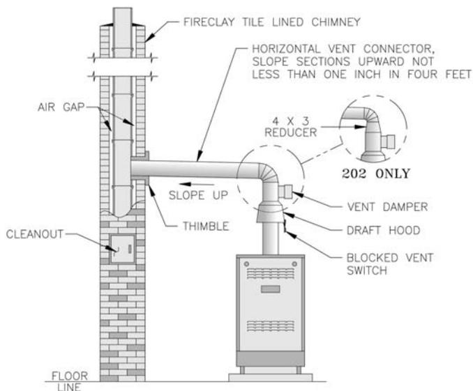
**Figure 8: Typical Vent Installation**
