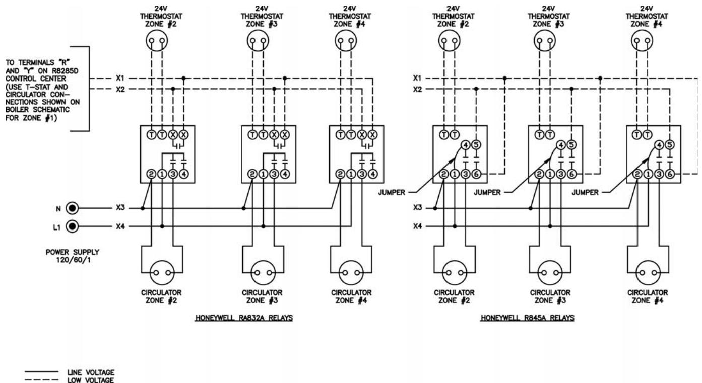
Figure 16: Wiring Schematic, Zone Circulators
