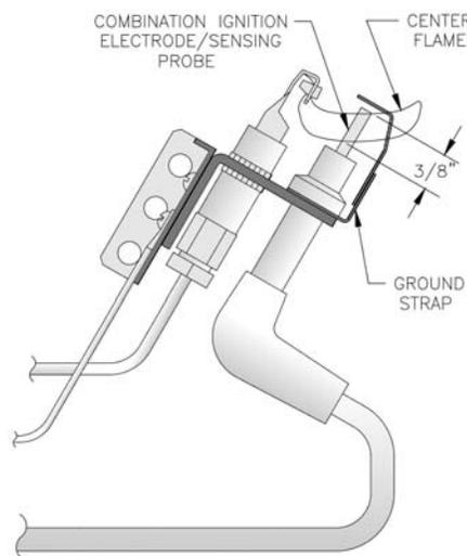
**Figure 26: Typical Pilot Flame, Honeywell Q348A**
