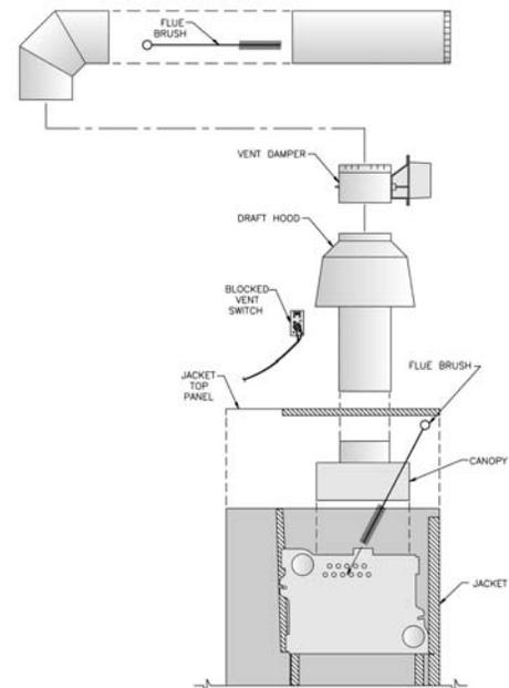
**Figure 28: Cleaning of Vent System and Boiler Flues**
