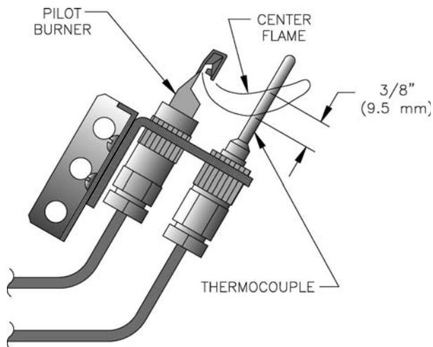
**Figure 25: Typical Pilot Flame, Honeywell Q327**
