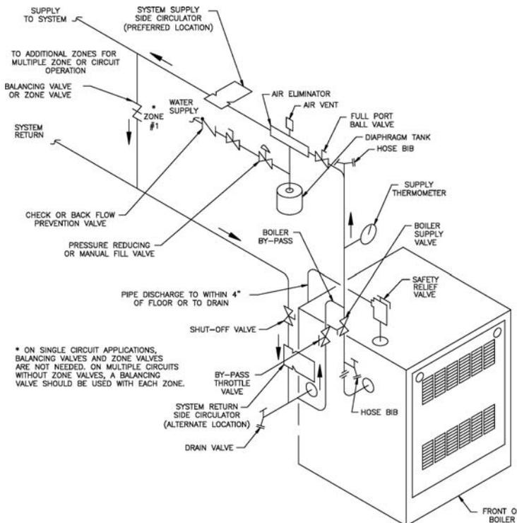
**Figure 3: Boiler Water Piping**
