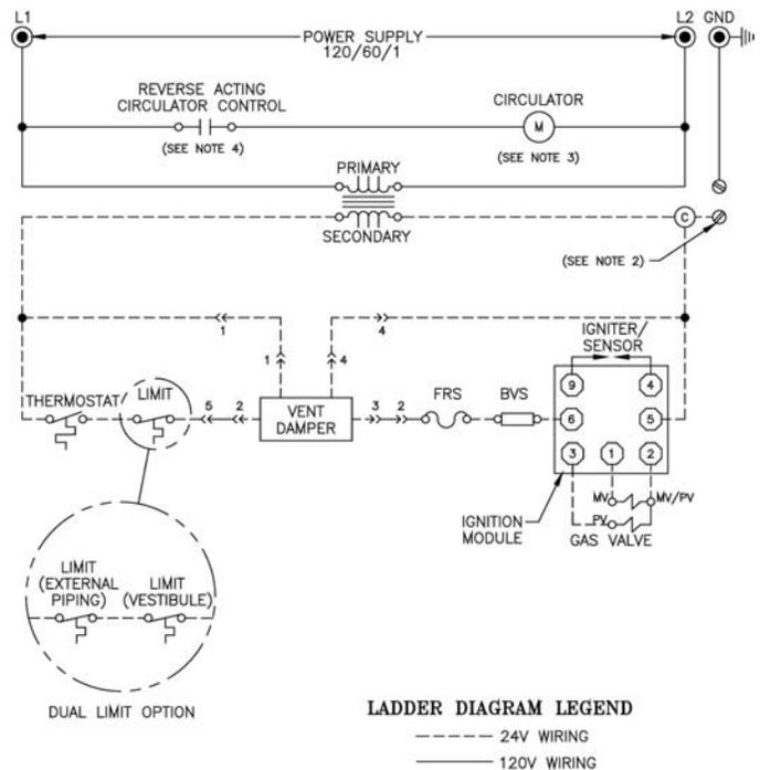
**Figure 14: Wiring Diagram, Electronic Ignition (EI), Continuous or Gravity Circulation**
