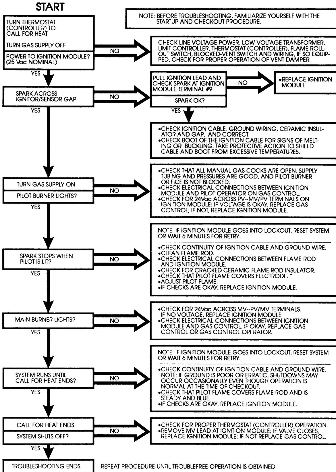
Figure 27: Troubleshooting Guide, Honeywell Electronic Ignition (EI)
