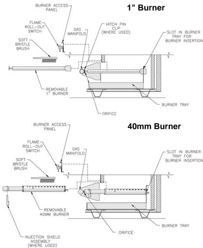
**Figure 29: Burner Cleaning and Installation**
