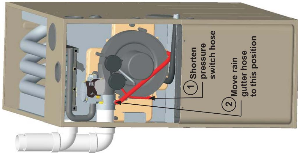
**INDUCER ROTATED FOR LEFT SIDE VENTING**
