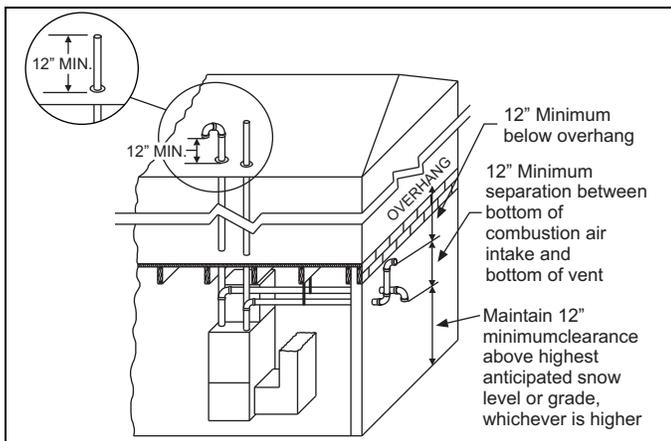
**FIGURE 27:** Termination Configuration - 2 Pipe Basement
