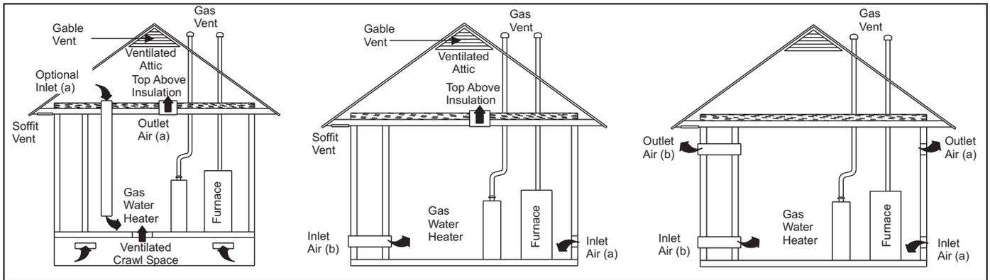
**FIGURE 32:** Outside and Ambient Combustion Air
