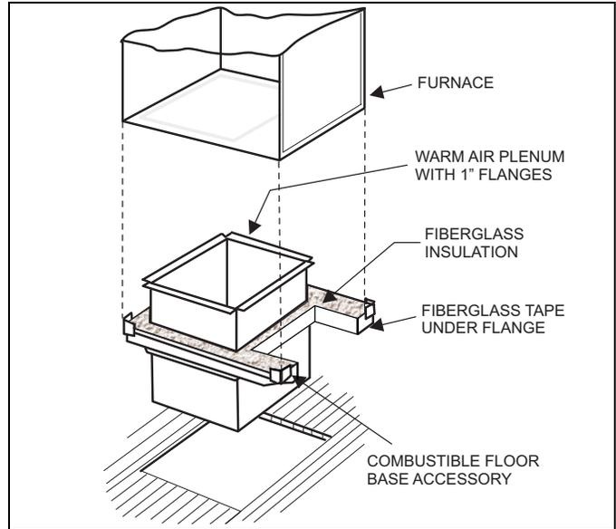
**FIGURE 10:** Combustible Floor Base Accessory
