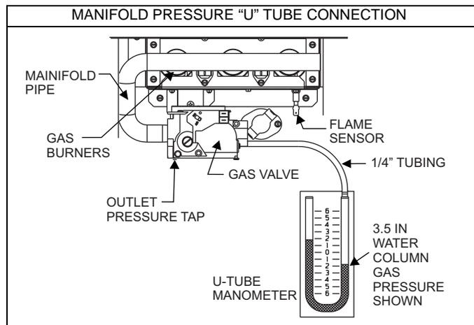
**FIGURE 35:** Reading Gas Pressure
