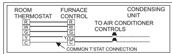
**FIGURE 18:** Single Stage Heat Thermostat Connections
