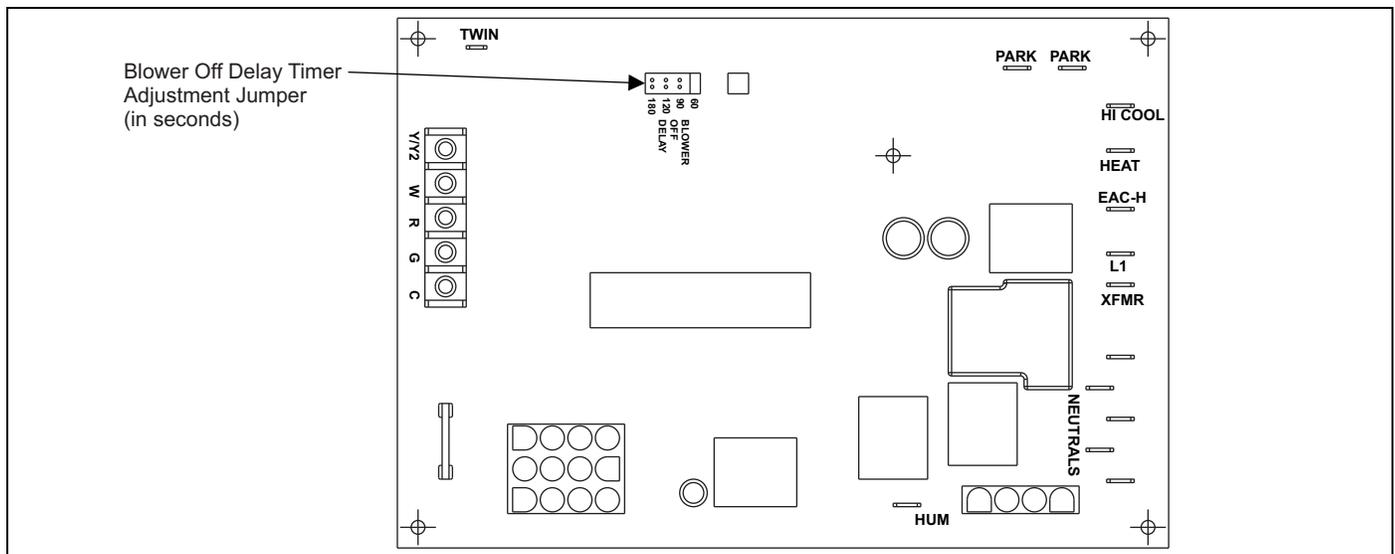
FIGURE 36: Furnace Control Board
