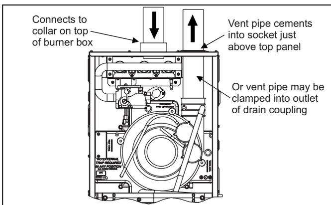
**FIGURE 31:** Direct Vent Air Intake Connection and Vent Connection
