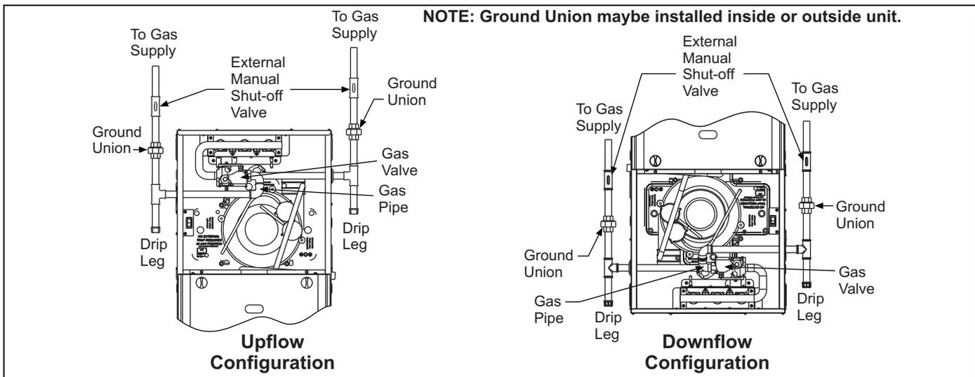
FIGURE 15: Upflow/Downflow Gas Piping
