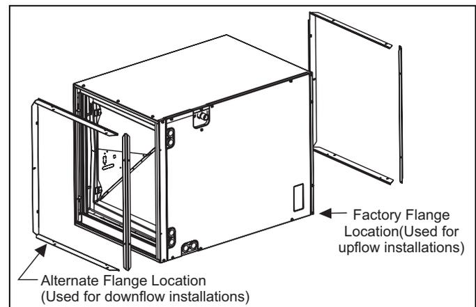
FIGURE 8: Coil Flange
