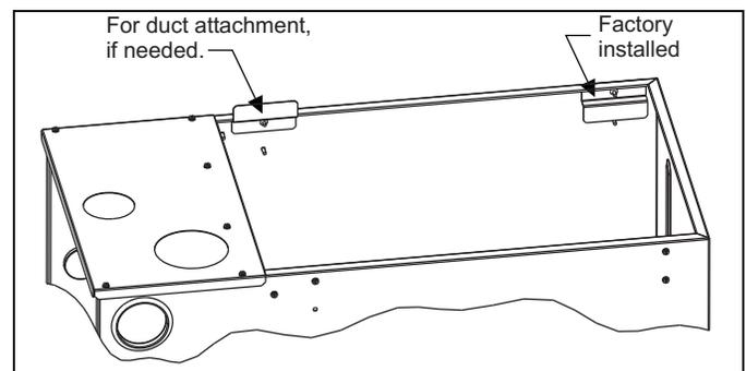
FIGURE 1: Duct Attachment
