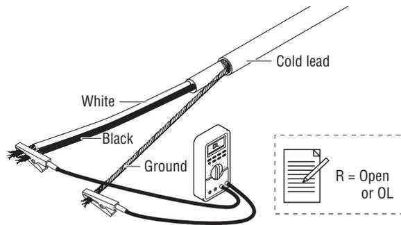
1. Connect the ground wire to the black lead and both power wires to the red lead of the multimeter.
