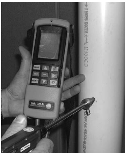
Figure 9.2: Insert Analyzer Test Probe into Test Port
