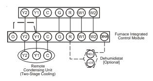
Thermostat - Two-Stage Heating with Two-Stage Cooling
