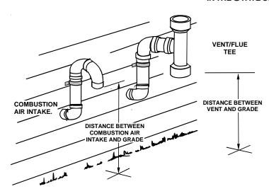
For all side wall horizontally vented gas fueled equipment installed in every dwelling, building or structure used in whole or in part for residential purposes, including those owned or operated by the Commonwealth and where the side wall exhaust vent termination is less than seven (7) feet above finished grade in the area of the venting, including but not limited to decks and porches, the following requirements shall be satisfied:
