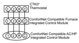
System Wiring using Four-Wires
