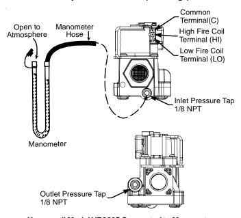
Honeywell Model VR9205 Connected to Manometer
