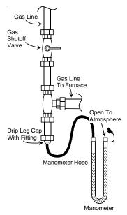
Measuring Inlet Gas Pressure (Alt. Method)
