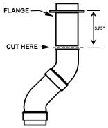
Vent/Flue Pipe Cuts
