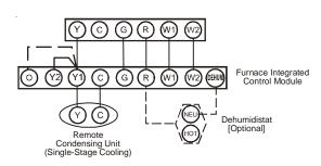
Thermostat - Two-Stage Heating with Single-Stage Cooling
