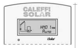
• With the air purged and flow rate set, set the control back into the Auto mode. If you forget to do this, the pump will continue pumping regardless of sensor temperatures.
