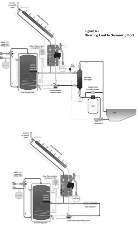
Figure 6.3 Diverting Heat to Dissipator
