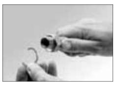
Slide on 1" union nut and close segment ring around pipe groove.
