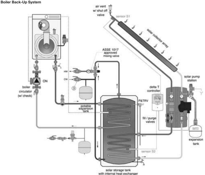
and boiler backup heat exchanger
