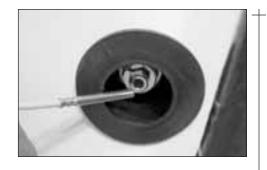
• Fasten temperature probe (the one having grey cord) into the bottom tank sensor well.
