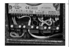
• Connect the other end of "J cord" into the controller. Connect the sensor wires. Consult the included *iSolar* controller installation instructions for more details on wiring controller.
