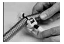
Cut pipe with tubing cutter. Do not use a hack saw.
