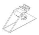
• With the lower brackets mounted onto the first panel, place the second panel (and then additional panels if applicable) into its respective mounting brackets and install mounting bolts through clips.
