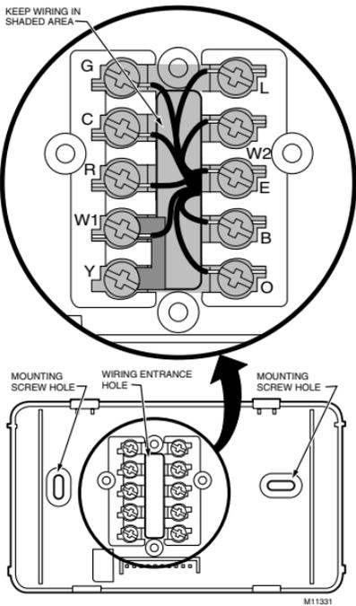
Fig. 4. Restrict wiring to shaded area.
