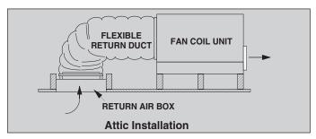
Same unit can be installed for horizontal or vertical supply air flow with simple field conversion.
