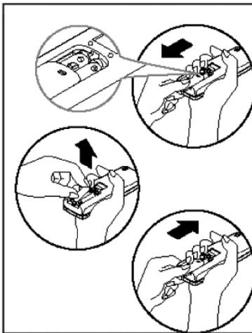
The remote controller is powered by two dry batteries (AAA 1.5V) housed in the rear housing and protected by a cover.
