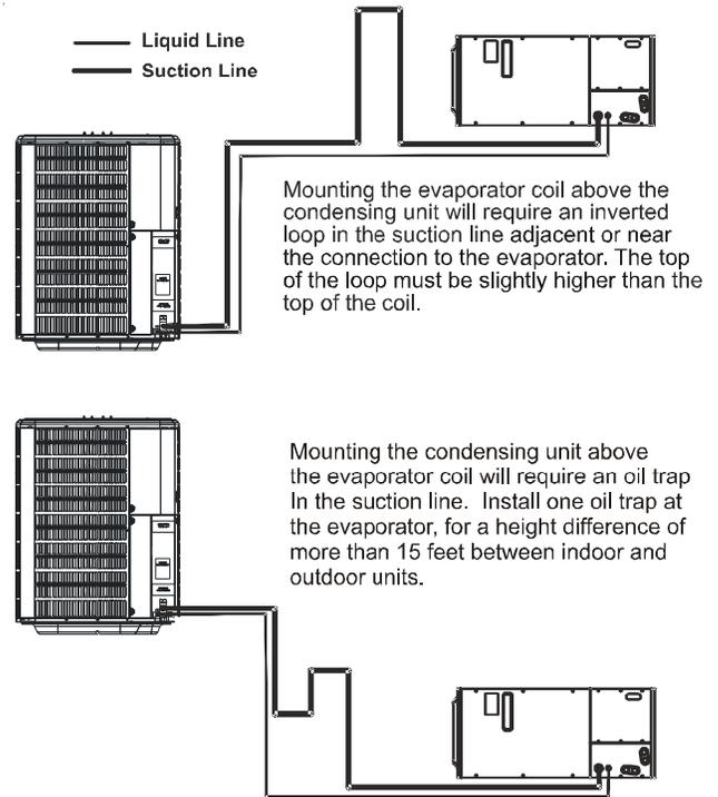
Insulation is necessary to prevent condensation from forming and dripping from the suction line. Armflex (or satisfactory equivalent) with 3/8" min. wall thickness is recommended. In severe conditions (hot, high humidity areas) 1/2" insulation may be required. Insulation must be installed in a manner which protects tubing from damage and contamination.
