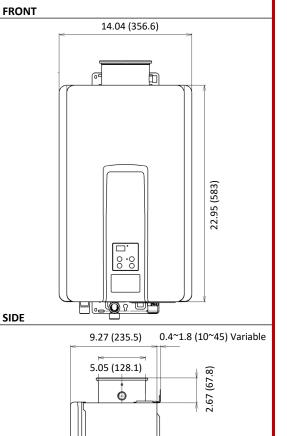
\* Clearance for servicing is 24 in. (610 mm) in front of water heater
