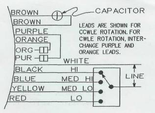
\*MOTOR CAN BE RUN WITH 5 OR 7 1/2 MFD/370 V CAPACITOR FOR 1/6, 1/5, 1/4, AND 1/3 HP RATINGS; HOWEVER, MOTOR IS APPROXIMATELY 10% STRONGER WITH THE 7 1/2 370 V CAPACITOR AND HAS HIGHER STARTING TORQUE.
