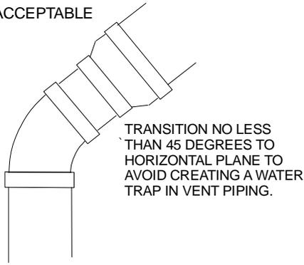
TRANSITION NO LESS THAN 45 DEGREES TO HORIZONTAL PLANE TO AVOID CREATING A WATER TRAP IN VENT PIPING.
