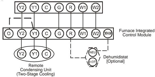
Thermostat - Two-Stage Heating with Two-Stage Cooling
