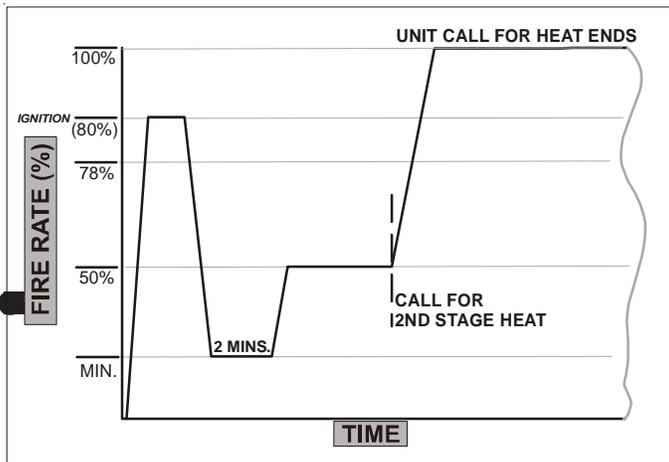
Call for 2nd-Stage Heat with 1st-Stage call for heat call in progress, with conventional 2-Stage Thermostat.
