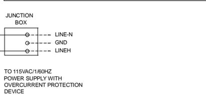
TO 115VAC/180HZ POWER SUPPLY WITH OVERCURRENT PROTECTION DEVICE
