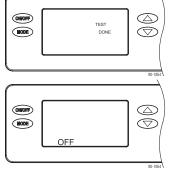
After one minute of compressor operation, all outputs will turn off and DONE will blink for 3 seconds and then return to the OFF screen.
