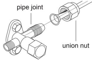
4. Tighten the union nut with torque wrench by referring to the sheet below.
