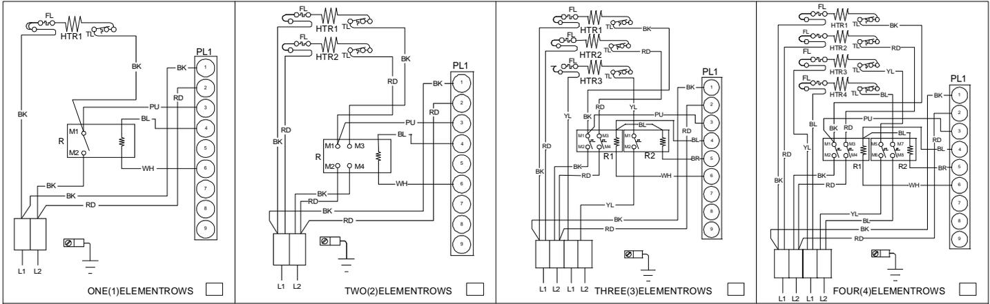
AFTER INSTALLING OPTIONAL HEAT KIT, MARK "X" IN THE PROVIDED ABOVE.
