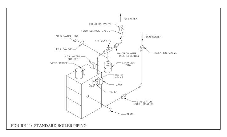
radiation. In addition, some codes such as ASME CSD-1 require low water cutoffs. Codes may also require that this low water cutoff have a manual reset function. The low water cutoff may be a float type or probe type, but must be designed for use in a hot-water system. The low water cutoff should be piped into the boiler supply just above the boiler with no intervening valves between it and the boiler.
