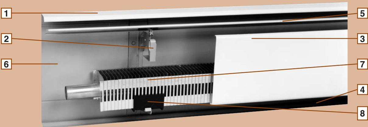
**1 - ENCLOSURE TOP AND BACK PANEL** - is of one-piece steel construction for strength and durability. Smooth surface won't collect dust and lint. Lower portion is extended 3/4" out from wall to cover any openings between wall and finished flooring and to let panel stand unaided while being fastened to wall.
