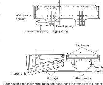
unit to the two bottom hooks while lowering the unit and pushing it against
