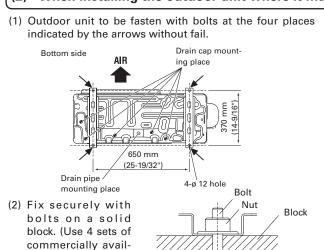
(3) Since the drain water flows out of the outdoor unit during heating operation, install the drain pipe and connect it to a commercial 16 mm (5/8") hose. (Reverse cycle model only) (4) When installing the drain pipe, plug all the holes other than the drain pipe mounting hole in the bottom of the outdoor unit with putty so there is no water leakage. (Reverse cycle model only)
