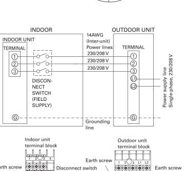
Power supply lin-Factory installed protective inline fuses for indoor units' conductors are installed on the Power Supply PCB.
