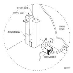
In a Single Zone — Not Ducted to HVAC System installation, the dehumidifier is not ducted to the HVAC system and is used to dehumidify a specific area. This installation is typically in basements or crawl spaces, with the dehumidifier ducted to the area requiring dehumidification.
