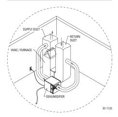
In a Single Zone — Ducted to HVAC System installation, the dehumidifier works in conjunction with the HVAC system, offering the optimum solution for year-round, wholehome control. This installation is typically in basement or attic locations. In a typical setup, air is pulled from the return duct, dehumidified, and returned to the return or supply duct. Alternate duct configurations are possible.
