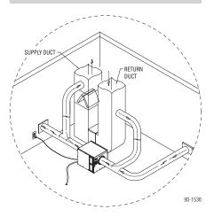
In a Two Zone — Primary and Secondary Zoned installation, the dehumidifier controls humidity in two zones. The dehumidifier will dehumidify the primary zone as the first priority, switching to the secondary zone after the primary zone dehumidification need has been met.
