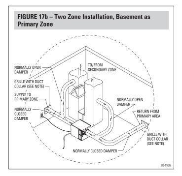
**Ducting Note:** The 1770A delivers approximately 500 CFM and the 1750A delivers approximately 275 CFM. Size ductwork and install multiple branches and grilles as needed to reduce airflow velocities to acceptable levels for the application.
