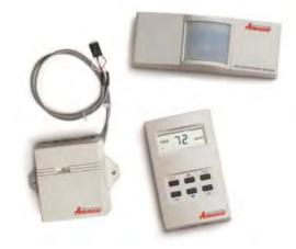
The DigiSmart Occupancy Sensor completes the in-room equipment. This infrared sensor can determine if the room is occupied or empty and when empty, signal the PTAC to adjust the temperature to save energy based on programmable setbacks.
