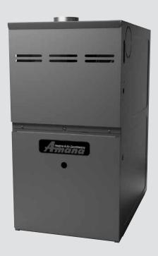
Amana® brand AMEH8 Upflow Horizontal, Two-stage Convertible, Multi-speed ECM Gas Furnaces feature a stainless-steel tubular heat exchanger and durable silicon nitride Ignition system. With a heavy-gauge reinforced, insulated steel cabinet and durable baked enamel finish, this unit can be installed in a variety of locations.
