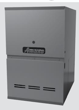
Amana® brand ADSH8 Downflow Horizontal, Two-stage Convertible, Multi-Speed Gas Furnaces feature a stainlesssteel tubular heat exchanger and durable silicon nitride Ignition system. With a heavy-gauge reinforced, insulated steel cabinet and durable baked enamel finish, this unit can be installed in a variety of locations.
