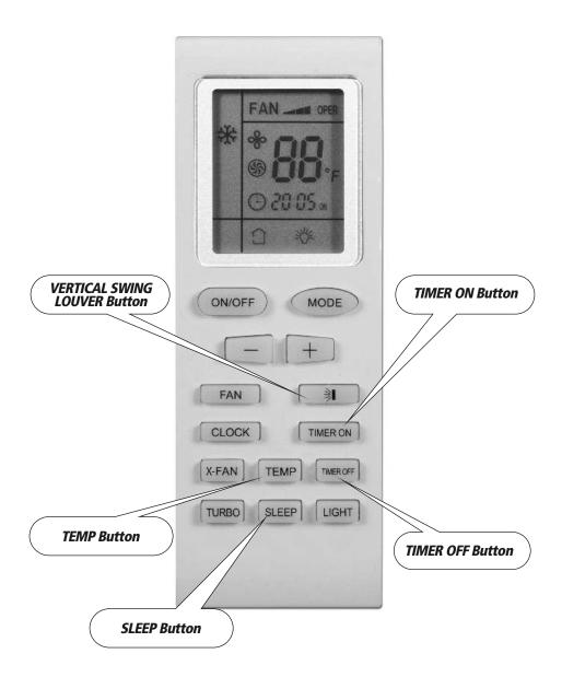
The wireless remote controller is the interface between the user and the neo system. Commands are entered by the user to control the system. Any command that has been entered with the remote controller will remain in memory until it is changed by the user or the batteries are replaced.
