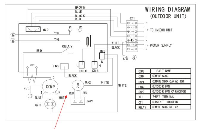
Note: This wire is BLUE in the outdoor unit using 208-230V power supply.
