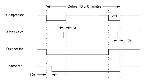
Remark: when the evaporator pipe temperature sensor more than TE16, the indoor fan start to run.
