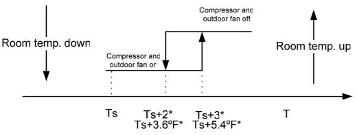
\* This parameter can be changed from 0 to 3°C (0 to 5.4°F).
