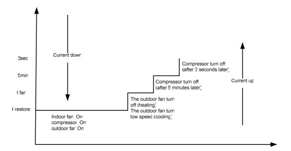
If compressor turns off for continuously 4 times due to current protection in 5 minutes from Compressor On, the unit stops and LCD displays failure information and can't returns to normal operation automatically.
