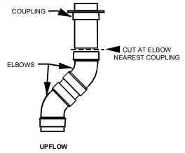
Vent/Flue Pipe Cuts
