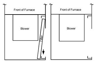
6. Replace filter by reversing procedure.
