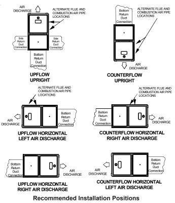
**NOTE:** Alternate "vertical" piping connections can not be used when an upflow furnace is installed with supply air discharging to the right, or when a counterflow furnace is installed with supply air discharging to the left. In either case, use the standard flue and combustion air piping connections.
