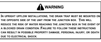
Follow the bullets listed below when installing the drain system. Refer to the following sections for specific details concerning furnace drain trap installation and drain hose hook ups.
