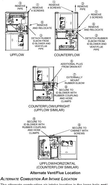
The alternate combustion air intake location is the large hole *not* in line with the induced draft blower outlet. To use the alternate combustion air intake location, refer to the following steps, and the "Alternate Combustion Air Intake Location" figure.
