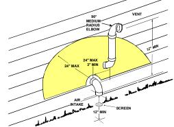
Alternate Horizontal Vent Termination (Dual Pipe)
