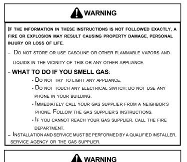
Should overheating occur or the gas supply fail to shut off, turn off the manual gas shutoff valve external to the furnace before turning off the electrical supply.
