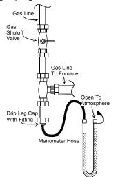
Measuring Inlet Gas Pressure (Alt. Method)
