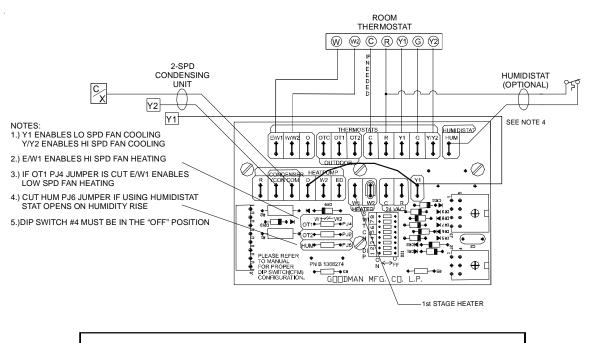
2 SPD COOLING ONLY - WITH 2 STAGE HEAT THERMOSTAT
