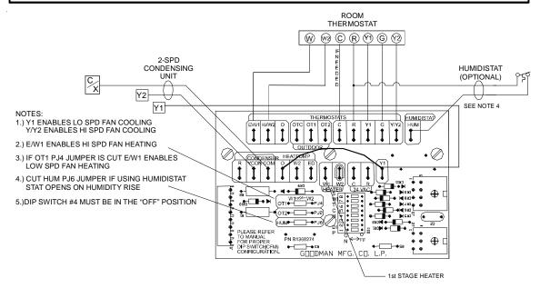
2 SPD COOLING ONLY - WITH 2 STAGE HEAT THERMOSTAT
