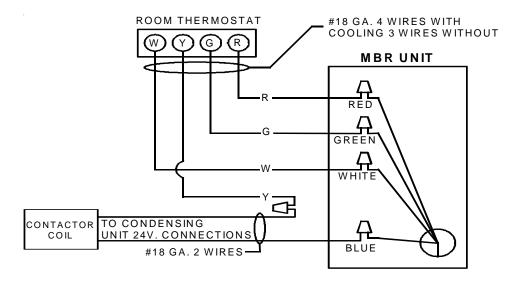
Figure 7- Low Voltage Wiring Diagram for Cooling Unit with optional heat kit 10KW and below
