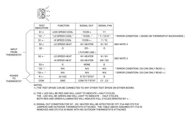
The chart above provides troubleshooting for either version of the encoded thermostat option. This provides diagnostic information for the GMC CHET18-60 or a conventional two cool / two stage heat thermostat with IN4005 diodes added as called out in the above section.
