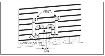
FIGURE 28: Double Horizontal Combustion Air Intake and Vent Termination
