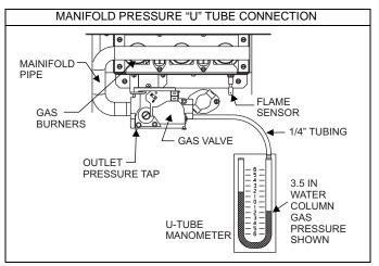
FIGURE 35: Reading Gas Pressure
