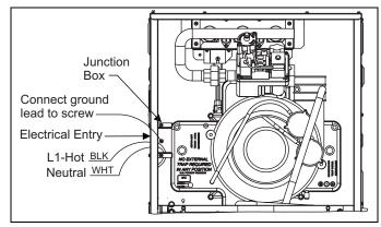
FIGURE 16: Electrical Wiring
