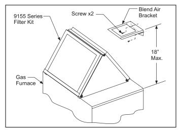
FIGURE 6: Blend Air Bracket
