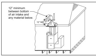
FIGURE 33: Attic and Crawl Space Combustion Air Termination
