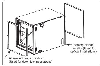
FIGURE 8: Coil Flange
