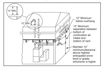
FIGURE 27: Termination Configuration - 2 Pipe Basement
