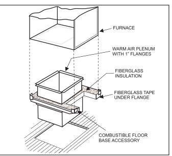
FIGURE 10: Combustible Floor Base Accessory
