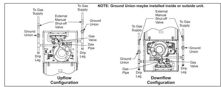
FIGURE 15: Upflow/Downflow Gas Piping
