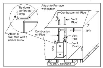
FIGURE 2: Attachment to Structure
