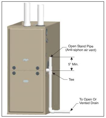
FIGURE 20: Typical Condensate drain, vertical installation
