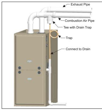
FIGURE 21: Typical Combustion Pipe Drain Tee
