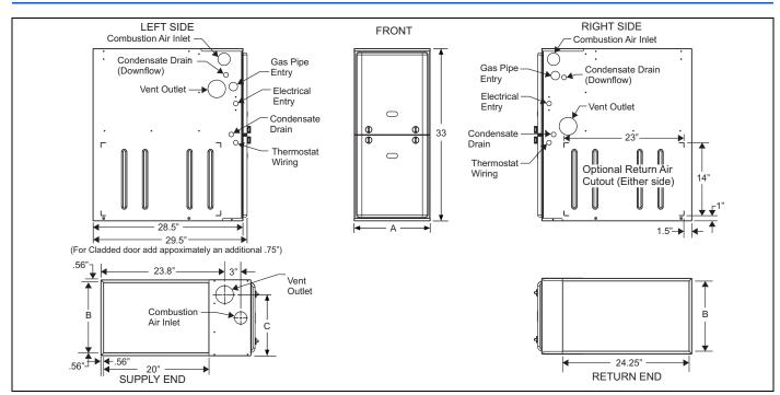
FIGURE 12: Dimensions (Upflow configuration shown)
