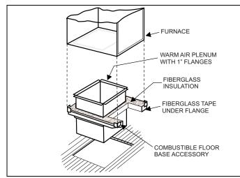
FIGURE 3: Combustible Floor Base Accessory
