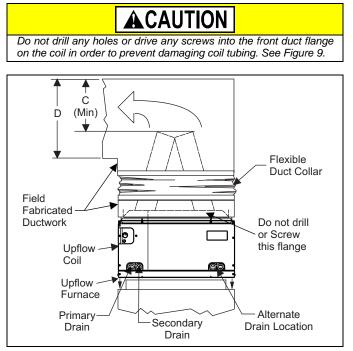
FIGURE 9: PC Series Upflow Coil Installation
