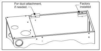
FIGURE 1: Duct Attachment
