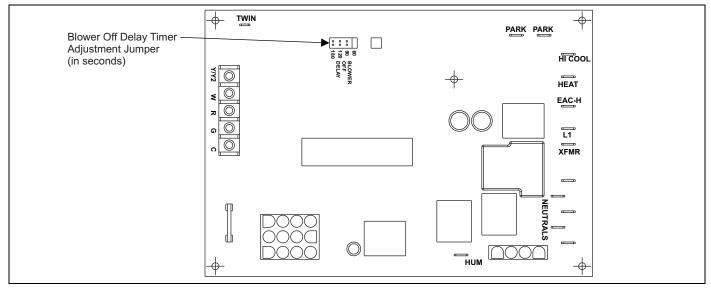
FIGURE 36: Furnace Control Board
