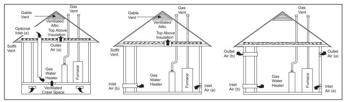
FIGURE 32: Outside and Ambient Combustion Air
