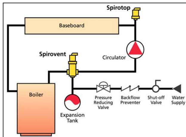
*Figure 1 Heating System*
