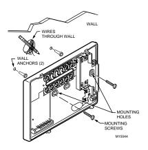
Fig. 2. Mounting the wallplate.
