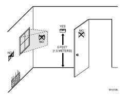
Fig. 1. Typical location of thermostat.
