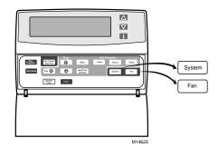
Fig. 9. Thermostat System and Fan key locations.
