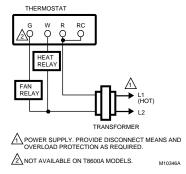
Fig. 3. Typical hookup in heat only application.
