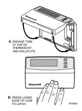
Fig. 7. Mounting thermostat on wallplate.
