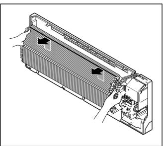
• Unhook the tab on the right inside of the chassis at the same time, slightly pull the evaporator toward you until the tab is clear of the slot.
