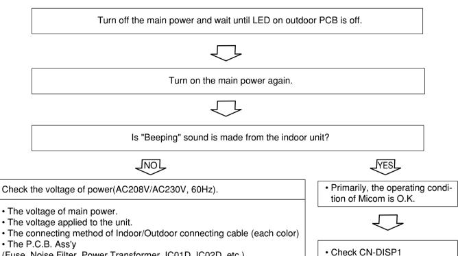
(Fuse, Noise Filter, Power Transformer, IC01D, IC02D, etc.)
