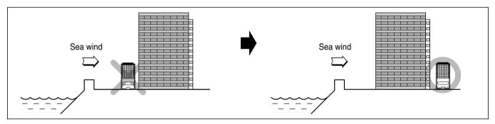
2) To install the outdoor unit on the seaside, set up a windbreaker/barrier to keep the unit from being exposed to the sea wind.
