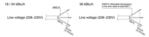
The power connecting cable connected to the indoor and outdoor unit should comply with the following specifications: ETL recognized and CSA certified.
