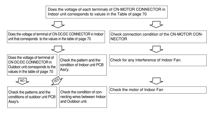
\* Indoor Fan may be off in the Soft Dry Mode(change to the Cooling Operation Mode).
