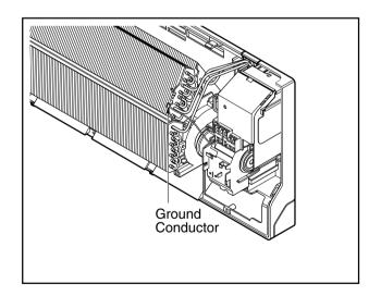
1. Before removing the control box, be sure to take out the wire screwed at the other end.
