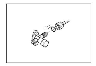
Finally, tighten the flare nut with torque wrench until the wrench clicks.
