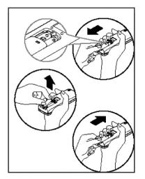
The remote controller is powered by two dry batteries (AAA 1.5V) housed in the rear housing and protected by a cover.
