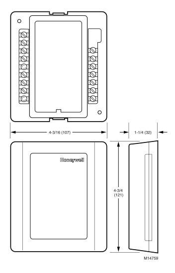
Fig. 1. W8703A dimensions in in. (mm).
