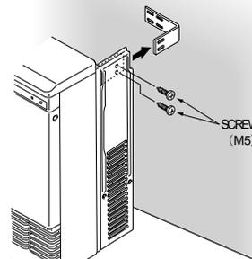
6. Attach the back spacer with 3 screws to the top of the appliance.
