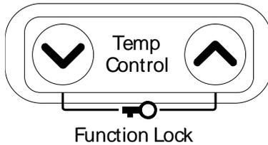
If the Lock is engaged while the unit is operating, all buttons will be disabled except for the ON/OFF button.
