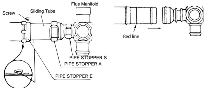
4. Slide the insulation sleeve up to the flue manifold and slip the securing clip over the sleeve as shown.
