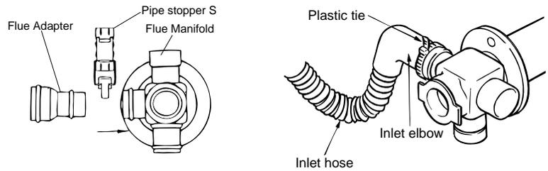
3. Connect the vent sliding tube with pipe stopper S and E. The sliding tube should not be extended beyond the red line. The red line should not be visible after sliding the tube into the vent outlet.
