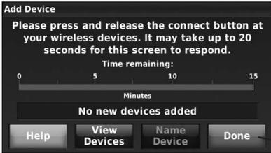
While the Add Device screen is displayed on the thermostat, **press and release** the **CONNECT** button on each wireless device, as described below. Accessories need to be at least 2 feet away from the thermostat during the linking process.
