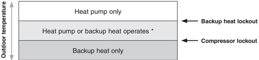
\* No backup heat unless indoor temperature drops to selected Backup Heat Differential setting, or Backup Heat Upstage Timer expires. **Heat pump turns OFF when backup heat turns on.**
