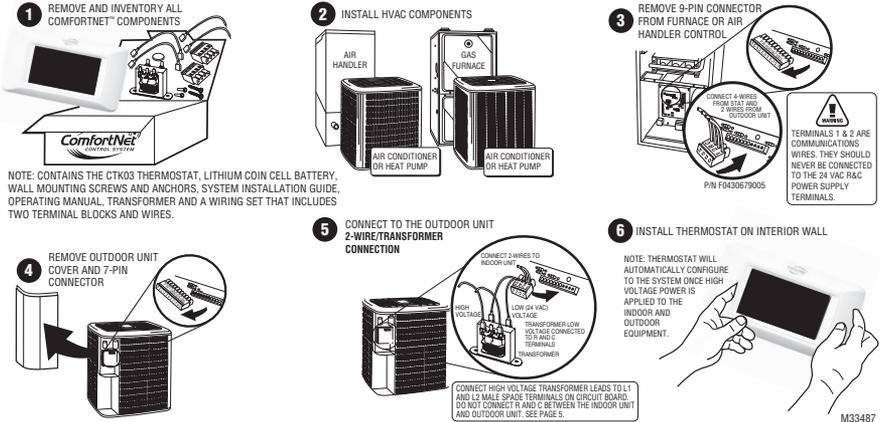
1. Remove and inventory all ComfortNet components. The box contains the ComfortNet CTK03 communicating thermostat, lithium coin cell battery, wall mounting screws and anchors, system installation guide, operating manual, transformer and a wiring set that includes two terminal blocks and wires.
