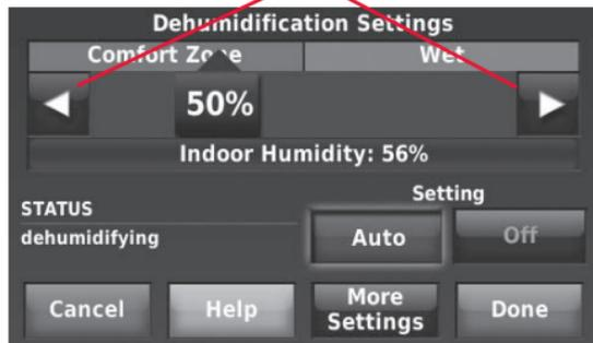
This feature can control your air conditioner to reduce humidity. Move the slider bar to the humidity level you prefer, then press **DONE**.
