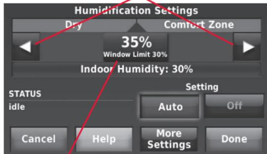
Window Protection limits the amount of humidity to prevent frost or condensation on windows
