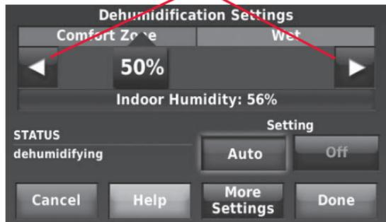
Move the slider bar to the humidity level you prefer, then press **DONE**. If your air conditioner is used to control humidity, the thermostat may use the following methods to maintain your desired humidity:
