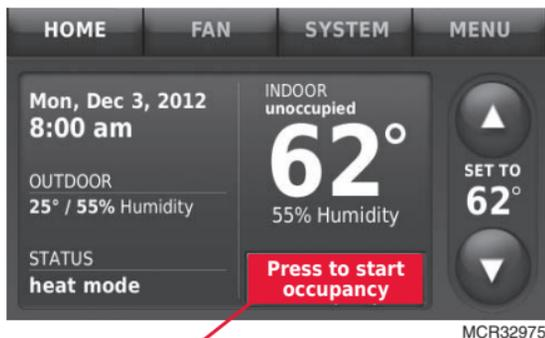
Press to maintain comfortable temperature while room is occupied
