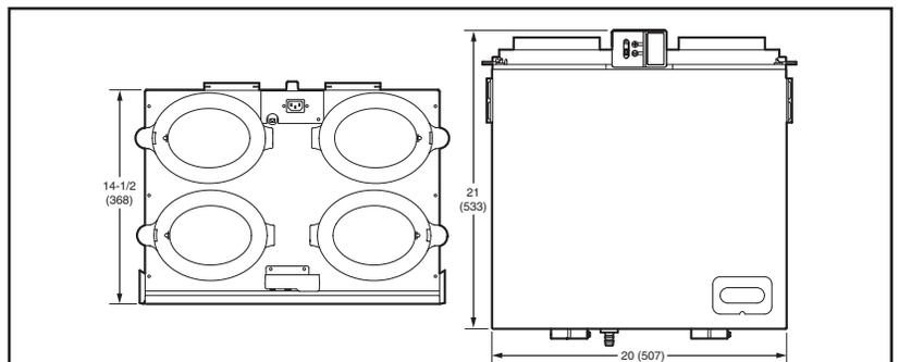
Fig. 1. Dimensions in in. (mm) and clearances.
