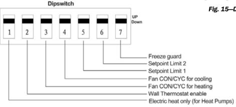
Fig. 16—Dipswitch Location on Unit
