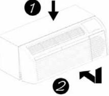
Place tabs over top rail (1). Push Inward at bottom until panel snaps into place (2).
