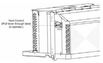
Fig. 12–Ventilaiton Control Location
