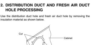
• Cut off the part (Cabinet) indicated by the arrow in the figure with
