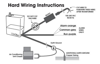
To install a ClearVueKübe Condensate Pump in applications where the supplied plug is not suitable, hard wiring may be necessary.
