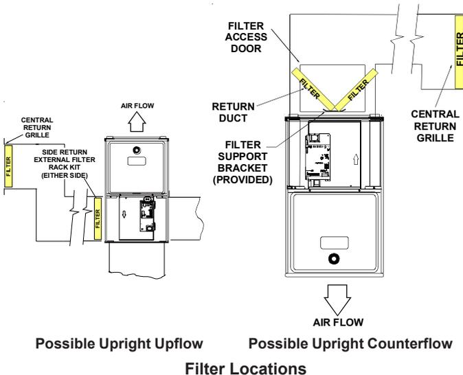
**NOTE:** Internal filter retention is not provided on this furnace. If an internal installation is desired, an internal filter retention kit is available as an accessory. Please see your distributor for details.
