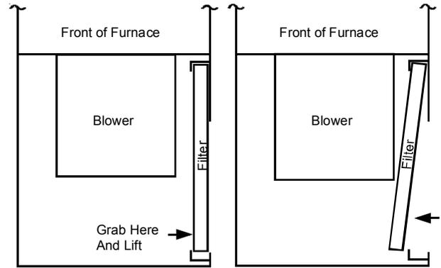
4. Angle filter toward the blower until filter clears bottom rail.
