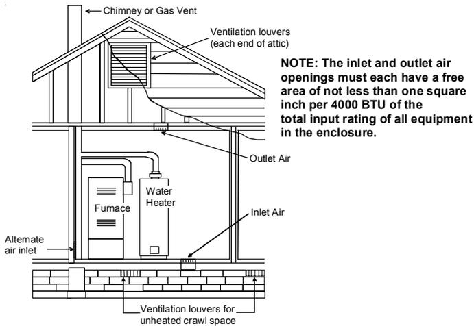
**Equipment Located in Confined Spaces; All Air from Outdoors—Inlet Air from Ventiladed Crawl Space and Outlet Air to Ventiladed Attic. See 5.3.3-b**
