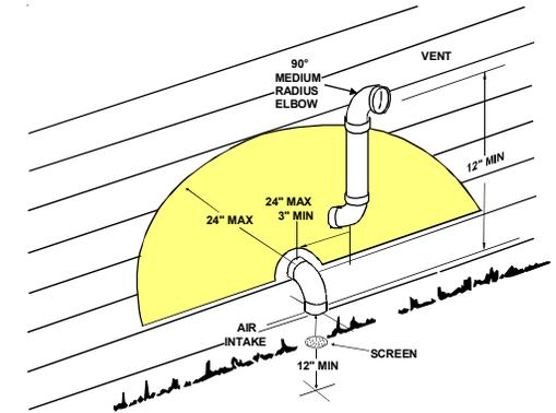
**Alternate Horizontal Vent Termination (Dual Pipe)**
