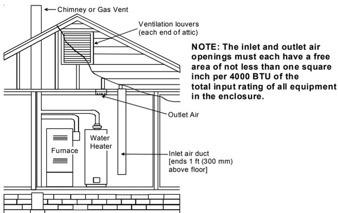
**Equipment Located in Confined Spaces; All Air from Outdoors Through Ventiladed Attic. See 5.3.3-b.**
