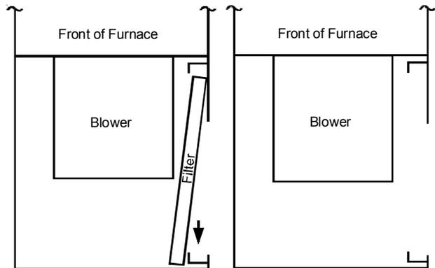
6. Replace filter by reversing procedure.
