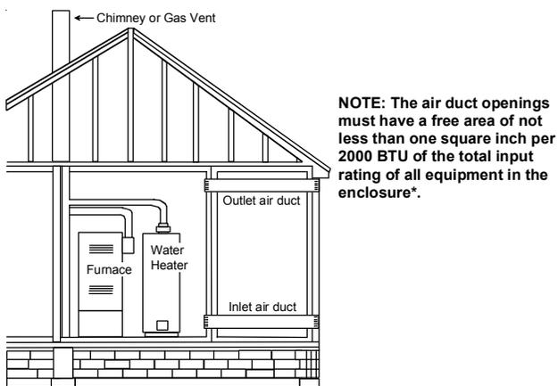
\*If the appliance room is located against an outside wall and the air openings communicate directly with the outdoors, each opening shall have a free area of not less than one square inch per 4,000 BTU per hour of the total input rating of all appliances in the enclosure.
