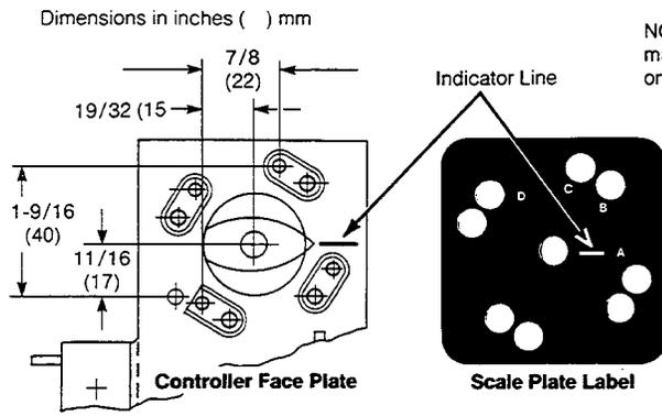
NOTE: Indicator line on label must align with indicator line on controller face plate.
