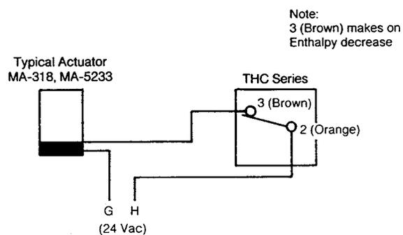
Figure-9 Economizer System with Two-Position Control.
