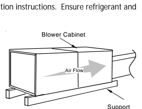
Figure 4 - Attic Installation
