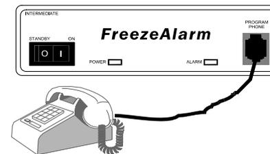
This phone will only be used to program your FreezeAlarm locally or for locally checking current status of your FreezeAlarm. It is important to UNPLUG this phone from the front after you are done programming or making any changes.
