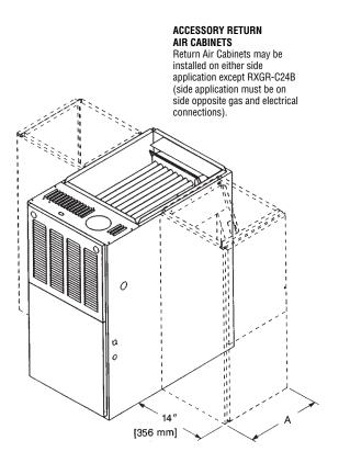
THE RXGR-C24B MAY ONLY BE INSTALLED ON THE SIDE OPPOSITE THE GAS AND ELECTRICAL CONNECTIONS.
