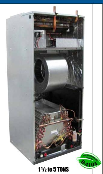
**HWCGxxX0A Series**– ECM constant torque blower motor is pre-programmed at the factory with speeds and torques controlled by software embedded in the motor for enhanced energy efficiency. Designed for use with a boiler loop, air handlers are AHRI matched to Heat Controller RSG split system condensers
