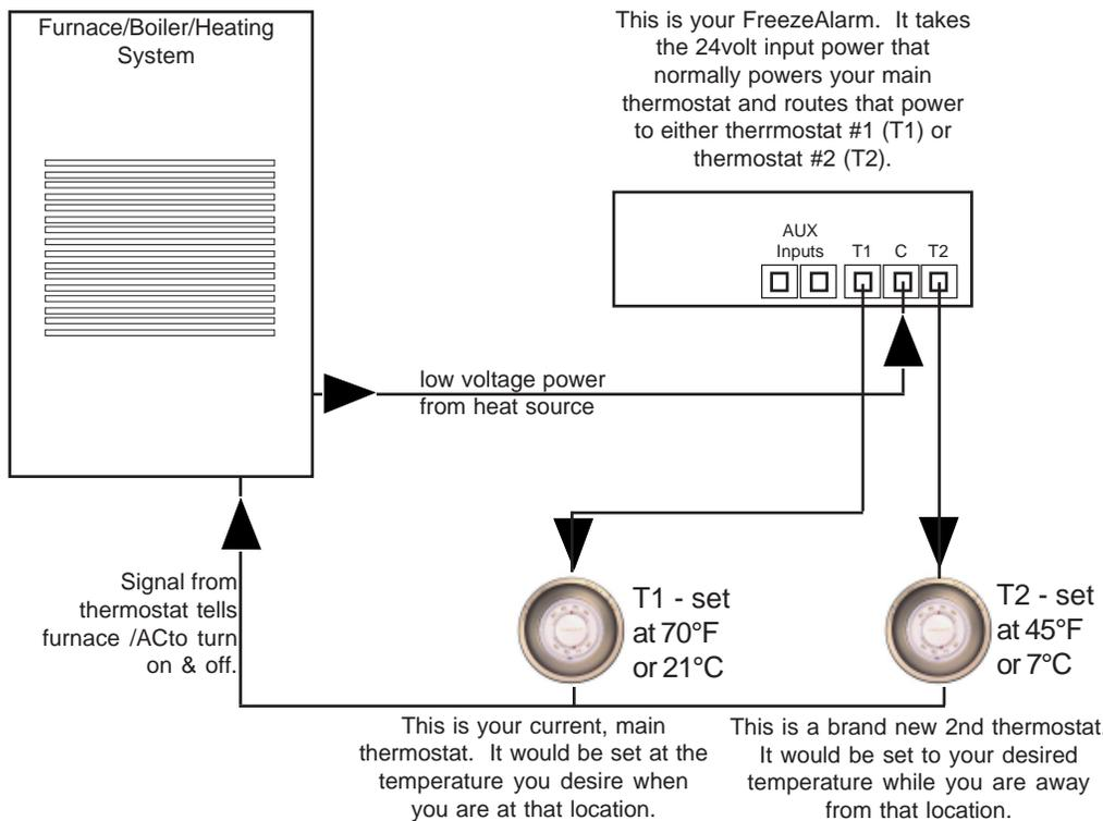
The diagram on the left shows how to wire your FreezeAlarm and Furnace or Heating System using LOW-VOLTAGE or MILLIVOLT thermostats only!
