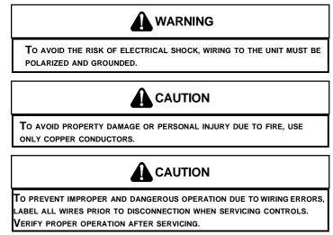
For unit protection, use a fuse or HACR circuit breaker that is in excess of the circuit ampacity, but less than or equal to the maximum overcurrent protection device. DO NOT EXCEED THE MAXIMUM OVERCURRENT DEVICE SIZE SHOWN ON UNIT DATA PLATE.
