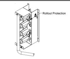
**Rollout Protection on Burner Bracket**
