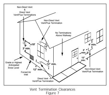
**NOTE:** In Canada, the current edition of CAN/CSA B149.1-15 takes precendence over the preceding termination restriction. **Special Venting Requirements For Installations In Canada**
