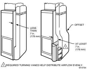
Fig. 13. Typical use of duct offset to make room for media air cleaner.
