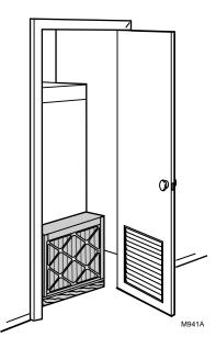
Fig. 5. Highboy furnace, with closet installation. Media air cleaner is mounted vertically on furnace between furnace and louvered return air opening in closet door.
