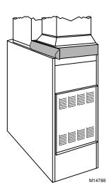
Fig. 6. Lowboy furnace, with media air cleaner mounted horizontally in return plenum just above furnace and opposite heating plenum.
